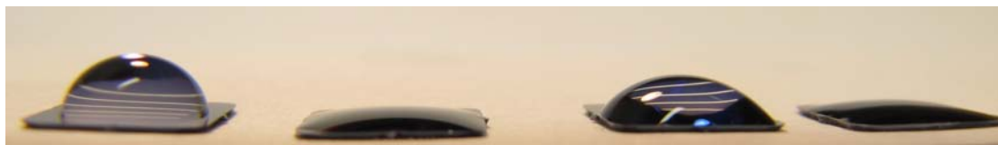
Figure 5-18. Water contact angles of (from left to right) an untreated ( 83^\circ ), oxygen plasma treated ( 14^\circ ), alumina-coated ( 56^\circ ), and alumina and oxygen plasma treated ( 18^\circ ) pnc-Si membrane chip.
