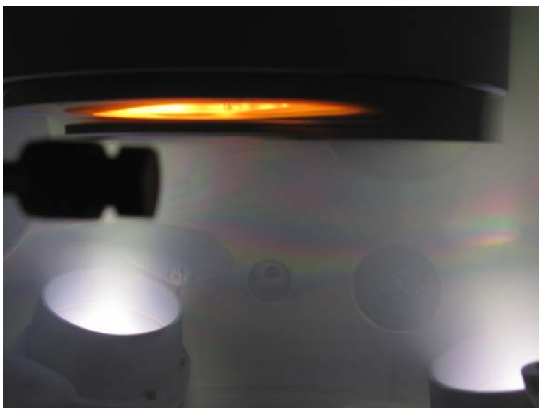
Figure 2-4. Physical vapor deposition by rf magnetron sputtering using a confocal target arrangement. The substrate is suspended from the rotation stage at the top of the image. The substrate may be heated via tungsten-halogen lamps to temperatures between room temperature and 800°C.
