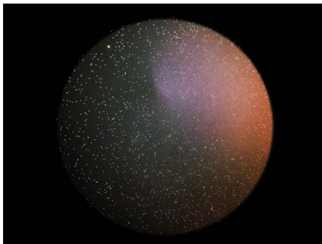
Figure 2-34. Dark field optical image of a film with a high density of particle contaminants. The particles act as scatterers, which appear as bright dots in the dark field imaging mode.
