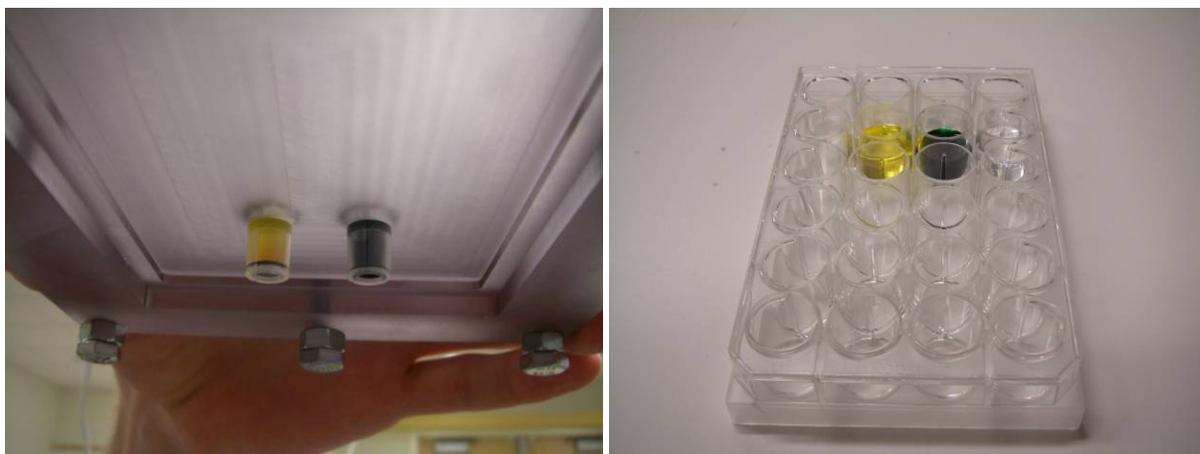
**Figure 15:** Right, the SepCons™ loaded with yellow and green dye were placed in the Nanomembrane Array device. Left, following pressurization of the device, the filtrate collection wells were observed to change color.
