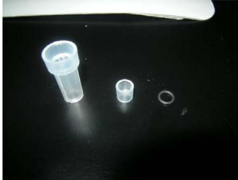
Three components of the SepCon™ are displayed above. From left to right, they are the housing cylinder, inner securing cylinder, and o-ring. The nanomembrane is not shown.
