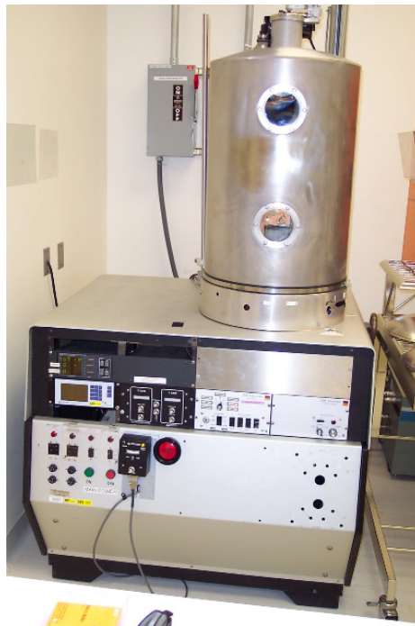
Figure 2.9: CHA e-beam evaporation tool.
