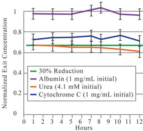
Figure 5: 12-hour clearance study. Exit concentrations normalized to inlet concentrations. Urea (4.1 mM), Cytochrome-C (1 mg/mL), and Albumin (1 mg/mL) in 100% serum were pumped through a single pass counter flow device. While the filter retained albumin, urea met its expected 30% reduction. Cytochrome-C (13 kDa) was also reduced.
