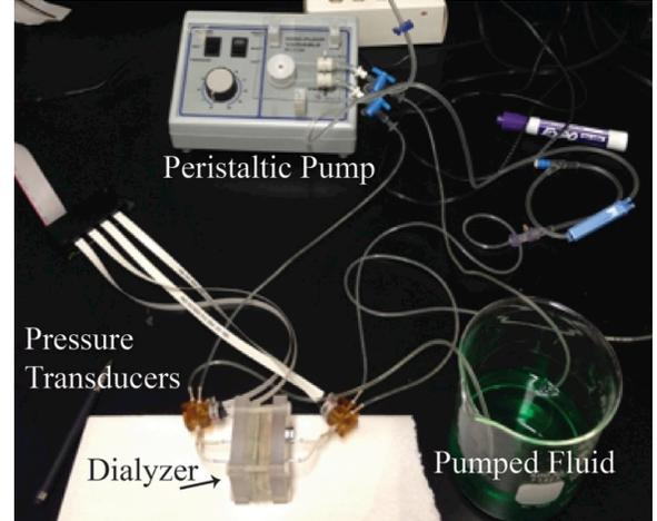
Figure 3: Flow pressure burst test setup. Peristaltic pump: 0.5 mL/min pumps fluid to and from beaker (at atmosphere) through ‘blood-side’ of the single chip dialyzer. ‘Dialysate-side’ is supplied via gravity feed.
