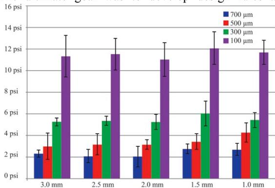
Figure 6: Burst pressures of rectangular membranes, lengths of 1.0 mm to 3 mm, and widths of 0.1 mm to 0.7 mm. Clearly, membrane width plays a more important role in determining the burst pressure than does lengths, for these dimension ranges.
