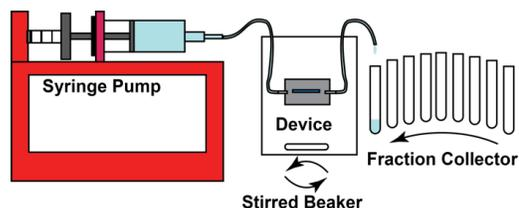
Figure 1: Long-term dialysis clearance set up. Syringe pump: 5 mL of 4.1 mM urea (or 1mg/mL Cytochrome-C and 1mg/mL Albumin), 5.6  $\mu\text{L}/\text{min}$ . Single channel dialyzer, 10 mm long, 0.5 mm wide. Fraction Collector programed to rotate every hour. Setup in refrigerator at 40  $^{\circ}\text{C}$ .
