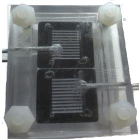
Figure 2: Two-chip dialyzer. ‘Blood-side’ shown, inlet from left divides fluid to both chips then evenly into the channels in the surface of the chips. Fluid was then collected from the channels and exits the single outlet on the right. Similar fluids route the dialysate across the smooth underside of the chip.
