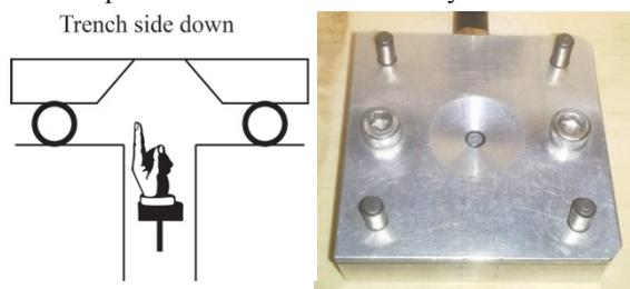
Figure 1: Static burst pressure setup. 5.4 mm chips were placed on the rubber o-ring over the compressed gas inlet port. The chip is held in place with an aluminum plate with an access hole that allows visual inspection of the membrane and acts as an outlet for the compressed gas after the membrane has burst. An electronic manometer recorded the burst pressure.
