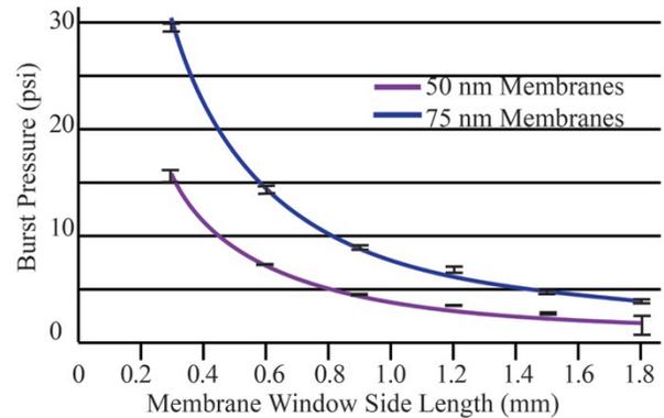
Figure 7: Static burst pressure results of 75 nm membranes vs. 50 nm membranes (square membranes). Burst pressures are doubled for a 1.5 fold increase in membrane thickness.
