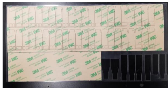
Figure 7: A laser cut sheet of polyester with adhesive pre-applied. Consistent strips can be made using this method, and they can be easily customized to fit certain dimensions.
