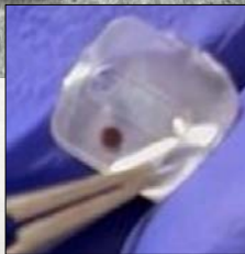
Grab flow insert with tweezers on smooth edges
